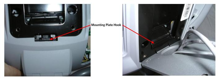
7. Disconnect the Data cable, Auto Stop cable (Treadmill only), Stop Key cable (Treadmill only), Hand Held HR Cable, Earth Ground wire and the Wireless HR Cable from the Upper PCA. **See Diagram 6.5.5.** Remove the console from the maintenance access hook and place it on a flat work surface.
