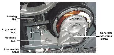
9. Set the replacement generator at its mounting position. Remove the three generator mounting screws, the two bearing clamp screws and the bearing clamp. Lift the generator and place the drive belt around the generator's pulley.
