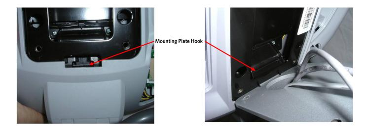
8. Disconnect the Data cable, Auto Stop cable (Treadmill only), Stop Key cable (Treadmill only), Hand Held HR Cable, Earth Ground wire and the Wireless HR Cable from the Upper PCA. **See Diagram 6.6.5.** Remove the console from the maintenance access hook and place it on a flat work surface.
