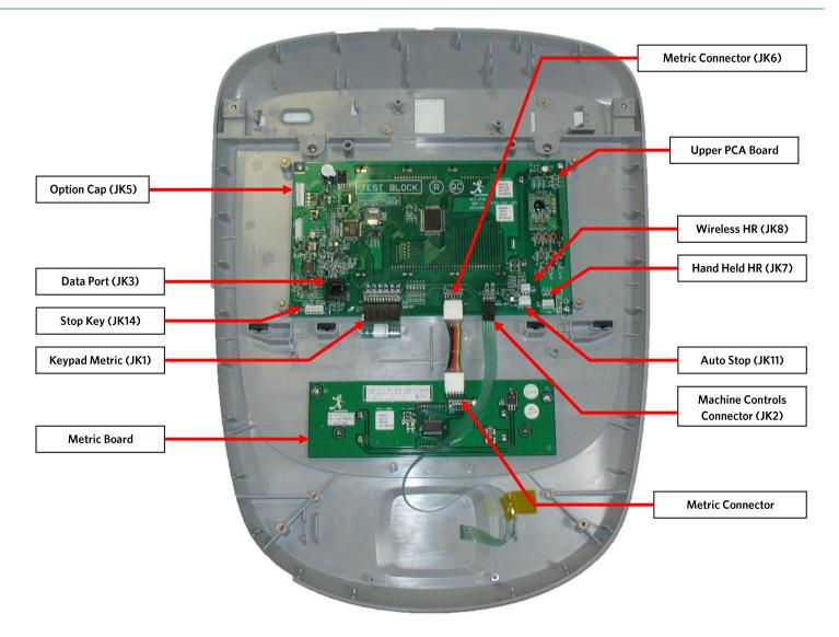
13. Install the replacement Metric PCA board into the console using the four screws removed in step 12. Torque to 10 inch pounds.
