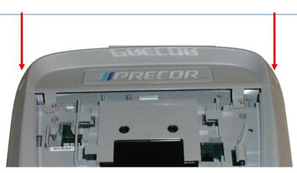
10. Remove the 6 screws that fasten the rear cover from the console and remove. See Diagram 6.6.7.
