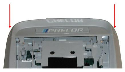
9. Remove the 6 screws that fasten the rear cover from the console and remove. See Diagram 6.5.7.
